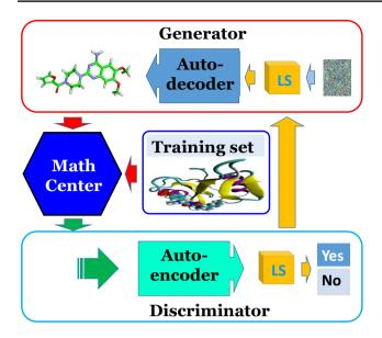
Fig. 5 Illustration of our docking approach using mathematical representations integrated with GAN architectures. The generator contains an autodecoder, a latent space (LS), and a noise source. The discriminator consists of an autoencoder and latent space. The Math center encodes 3D structures into low-dimensional mathematical representations using algebraic topology, differential geometry, and/or graph theory
